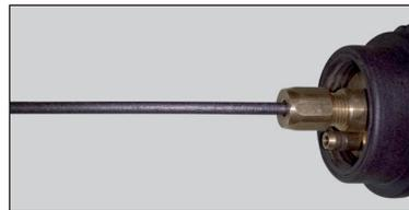
• Cut the carbon teflon liner protruding from the torch, so that the portion after the locking nut is exactly 3.75" (3 3/4").
