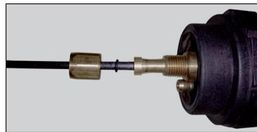
• On the liner protruding from the torch, insert the brass mandrel, the O-ring and the locking nut. The nut should be hand tightened. If it is too tight it may impede the feeding of the welding wire.
